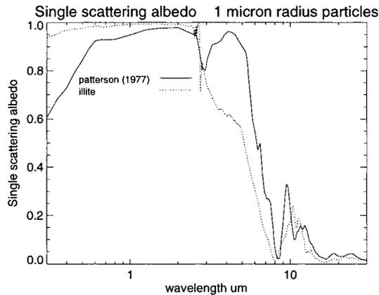
FIG. 1. Mie scattering calculations of single scattering albedo of 1- $\mu\text{m}$  particles assuming indices of refraction 1) from Patterson et al. (1977) as modified by Tegen and Lacis (1996) (solid line) and 2) for pure illite, Egan and Hilgeman (1979), and Querry (1987) (dotted line).
