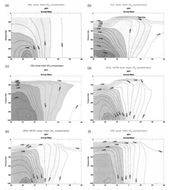
*Fig.* 6. Latitude-pressure cross-sections of annual mean simulated  $SF_6$  mole fraction (pptv) for 1993 for each model. The contour interval is 0.025 pptv, with shading thresholds at 2.875, 2.975, 3.075, and 3.175 pptv
