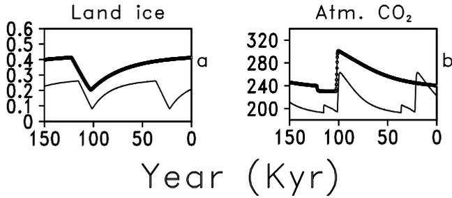
**Figure 8.** Results obtained with a different vertical mixing parameterization between southern box (VM\_S) with (thin line) and without (thick line) sea ice effect on air-sea flux. (a) Northern land ice extent as a fraction of polar land box area. (b) Atmospheric concentration of CO<sub>2</sub> (ppm).
