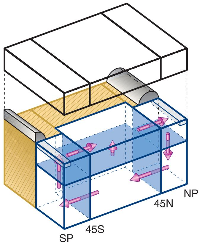
**Figure 1.** Schematic representation of coupled box model used in this study, showing atmospheric boxes (upper slab), thermohaline circulation (arrows), parabolic land ice sheets over land, and a partial sea ice cover in the polar ocean boxes. All of these physical climate system components are allowed to vary based on model equations. Ocean biogeochemistry and atmospheric CO<sub>2</sub> fully interact with physical climate components.
