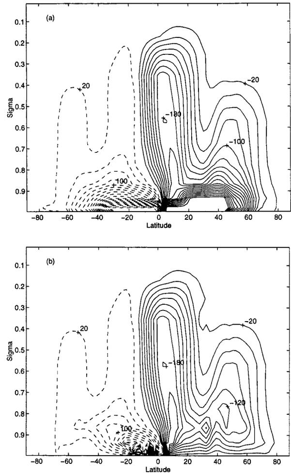
FIG. 3. Residual mean meridional streamfunctions [ $10^9 \text{ kg s}^{-1}$ ] corresponding to the isentropic mass circulation in Fig. 1: (a) conventional transformed Eulerian mean streamfunction  $\Psi_*$  and (b) modified residual streamfunction (hybrid of  $\Psi_*$  and  $\Psi_*^\dagger$ ).
