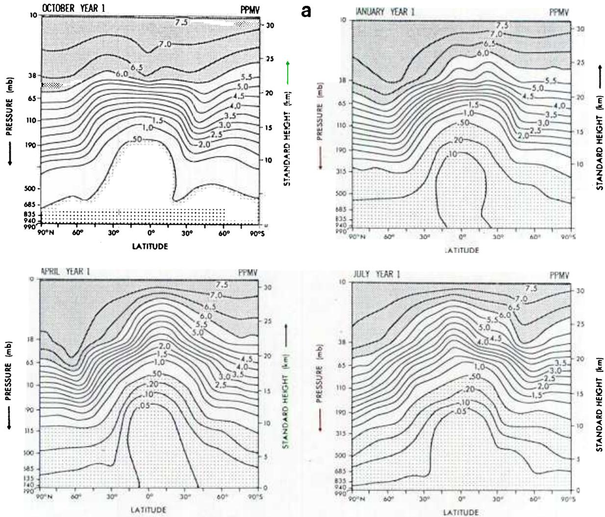
FIG. 3.2a. Zonal-mean mixing ratio (ppmv) for indicated months from the fourth year of the Stratified Tracer experiment. Note logarithmic contour interval within lighter shading.
