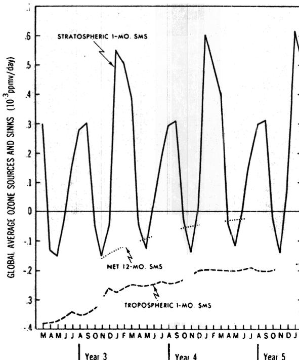
FIG. 5.5. Global average sources and sinks ( $10^{-3}$  ppmv day $^{-1}$ ) from the Simple Ozone experiment. Solid lines show stratospheric monthly mean net SMS averaged over the entire atmosphere. Dashed lines give monthly mean tropospheric destruction. The dotted line is the 12-month running mean of the net atmospheric SMS.
