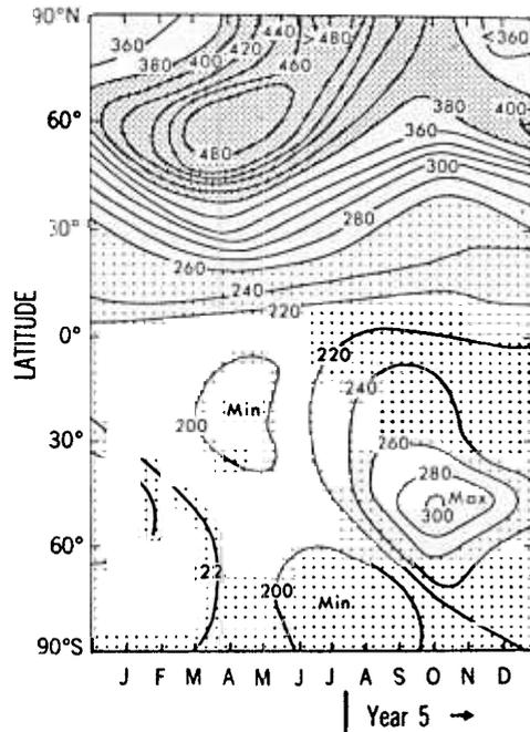
FIG. 4.3. Simulated zonal-mean total ozone ( $10^{-3}$  atm-cm) for 12 months of the year as simulated in the Simple Ozone experiment.
