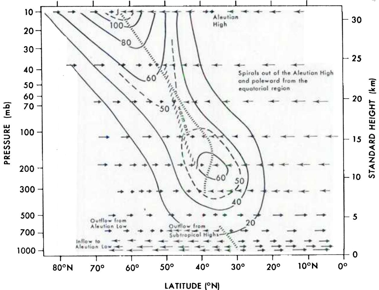
FIG. 5.7. Schematic view of net drift of all particles in the January-mean flow. Solid lines are isotachs ( $\text{m s}^{-1}$ ) at  $150^\circ\text{E}$ . Horizontal drift speed is roughly proportional to length of arrows. Actual drift is relative to time-mean flow axis, not latitude (see Fig. 5.6). Note position of strong convergence of particles (dashed lines) at and to the poleward side of the time-mean jet stream axis. The axis of warmest air is given by the diagonal dashed line.
