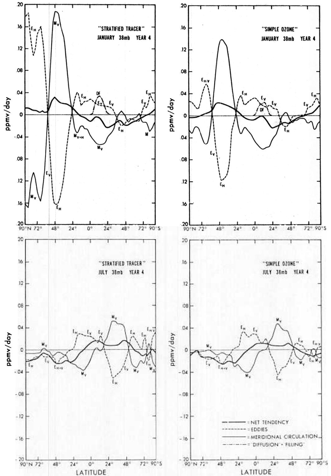
FIG. 5.4. 38 mb zonal-mean balances ( $\text{ppmv day}^{-1}$ ) for January and July from the Simple Ozone and Stratified Tracer experiments as indicated. Symbols as given in Eq. (5.1).
