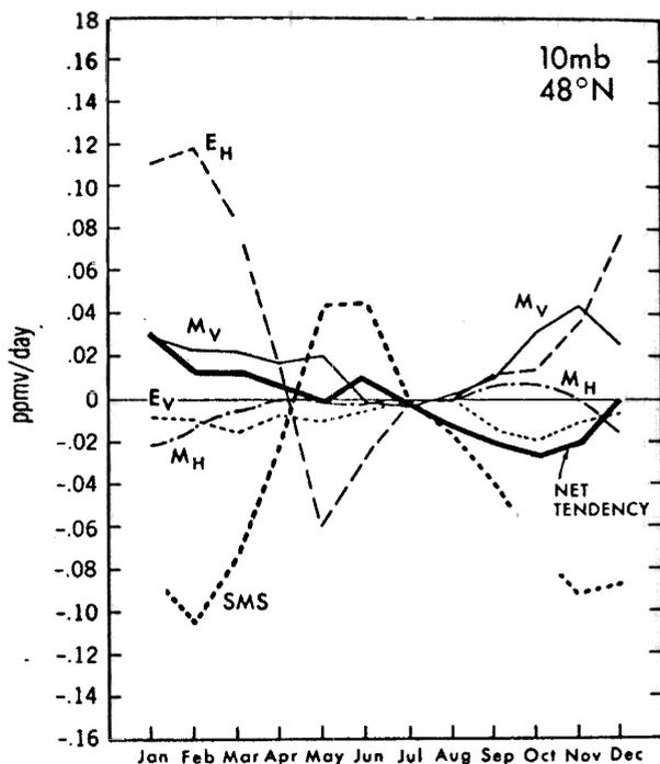
FIG. 5.2. Annual evolution of various contributions to the zonal-mean ozone balance ( $\text{ppmv day}^{-1}$ ) computed at 10 mb,  $48^\circ\text{N}$ . Symbols are as given in Eq. (5.1).
