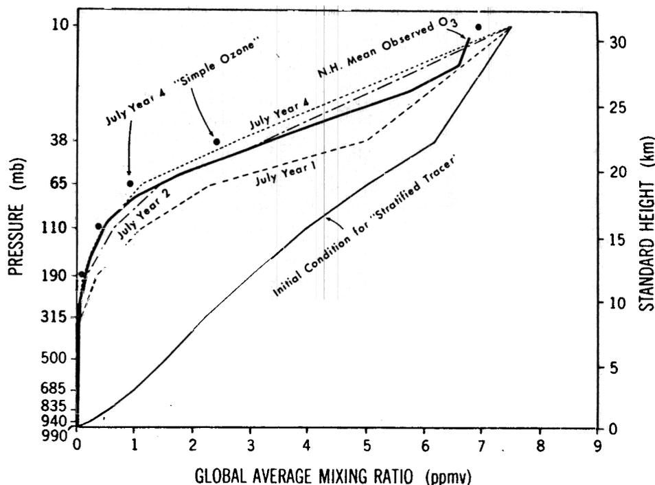
FIG. 3.1. Vertical distributions of the global-average mixing ratio from the Stratified Tracer experiment for the initial condition and July means of year 1, 2 and 4. Also shown are the Northern Hemisphere mean observed ozone [reanalyzed from Hering and Borden (1964, 1967)] and July year 4 from the Simple Ozone experiment (large dots).
