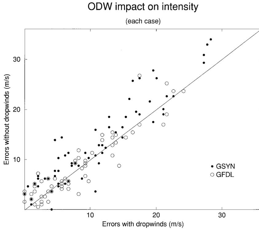
FIG. 14. Plot of individual GFDL model intensity forecast errors using analyses without vs with ODWs at 12, 24, 36, 48, and 72 h. Open circles and closed dots refer to experiments using NCEP synthetic vortex with and without the GFDL vortex specification system, respectively.
