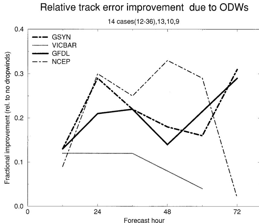
FIG. 8. The relative track error improvement due to ODWs for the GFDL model, the NCEP spectral model (T126 with synthetic vortex), and the VICBAR model. Fraction improvement is calculated as the difference in the track errors between model suites with and without ODWs normalized by the track error without ODWs. GFDL and GSYN refer to experiments using the NCEP synthetic vortex with and without the GFDL vortex specification system, respectively.
