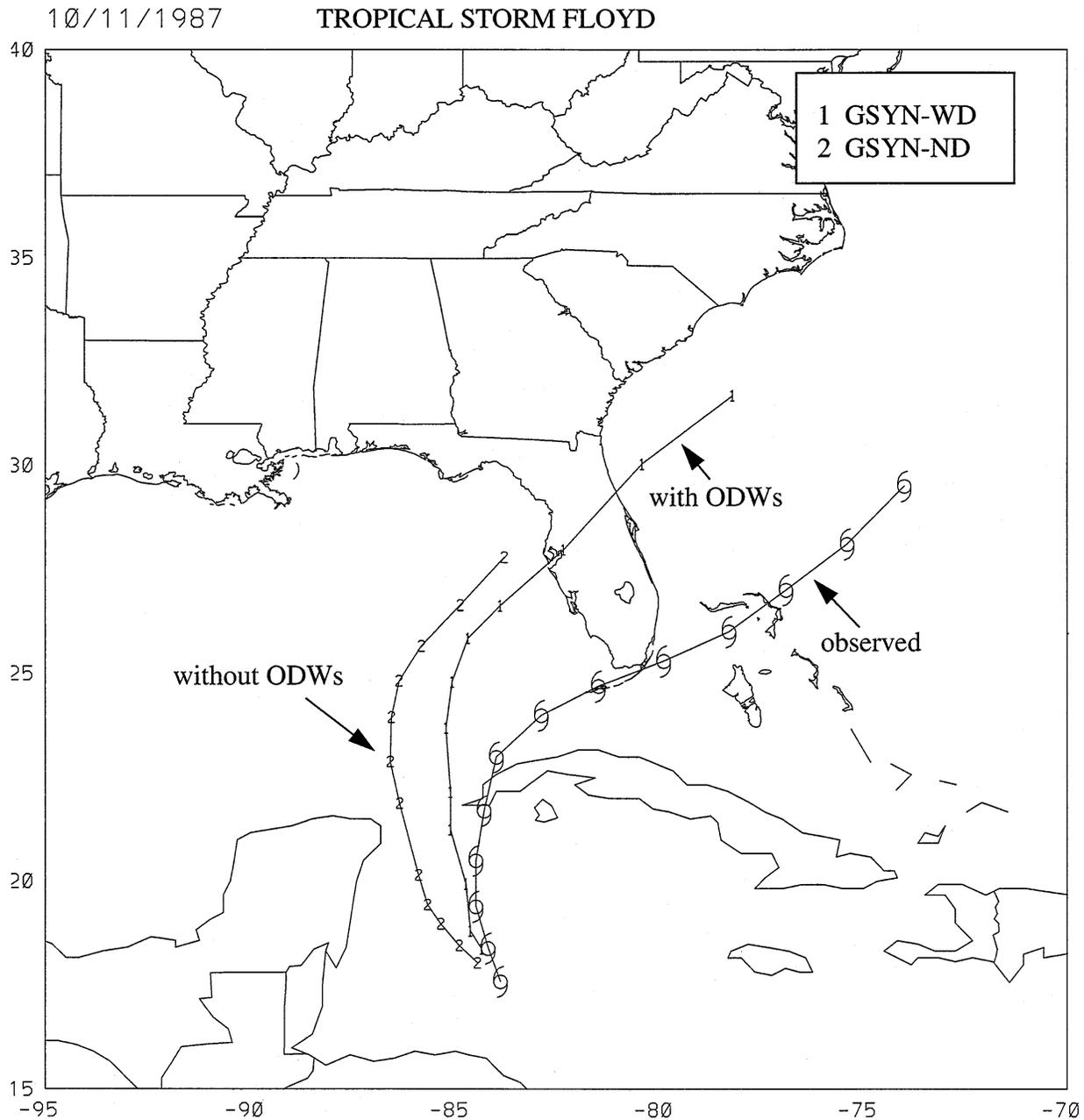
FIG. 9. Tracks of GFDL 3-day forecasts starting from 0000 UTC 11 October 1987 for Hurricane Floyd with and without ODWs ingested in the analyses. Results are for experimental series GSYN without the GFDL vortex specification system. The best track positions, including that at the initial time, are plotted with a tropical storm symbol, whereas the model forecasts are numbered and start at 6 h. Best track and model forecast positions are plotted every 6 h.
