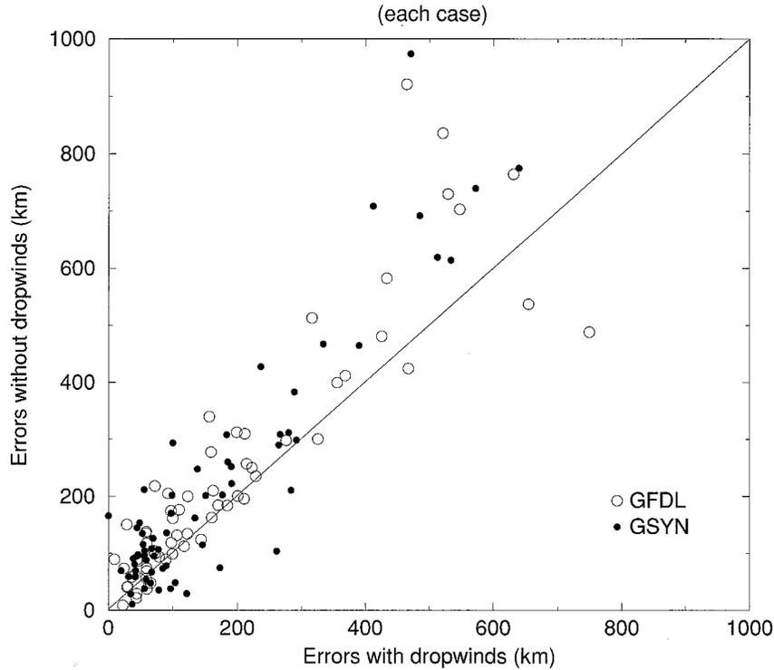
FIG. 7. Plot of individual GFDL model track forecast errors using analyses without vs with ODWs at 12, 24, 36, 48, and 72 h. Open circles and closed dots refer to experiments using NCEP synthetic vortex with and without the GFDL vortex specification system, respectively.
