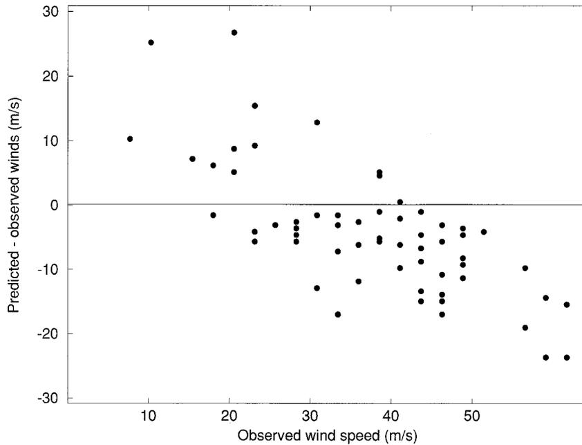
FIG. 5. A plot of the forecast intensity bias (predicted – observed) versus the observed wind speed for the GFDL suite of experiments for the 14 cases studied. Data are plotted for 12-, 24-, 36-, 48-, and 72-h forecast times.
