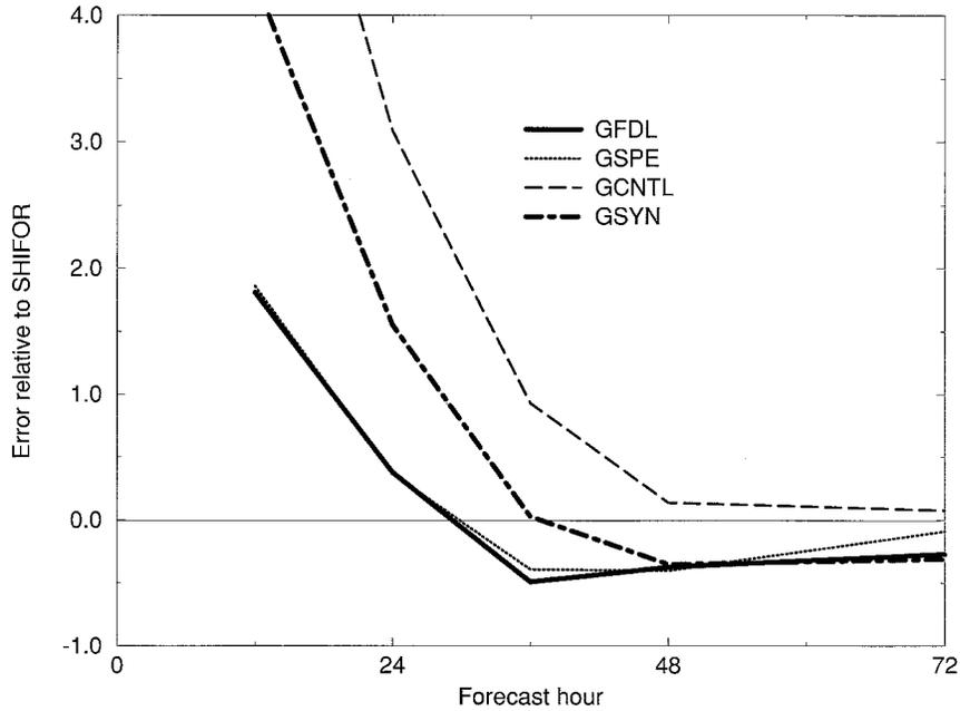
FIG. 4. Mean intensity errors for four modes of the GFDL model relative to SHIFOR for the 14 cases studied. Similar to the standard CLIPER diagram (Fig. 3), positive skill has negative values. The initial conditions used are those without ODWs.
