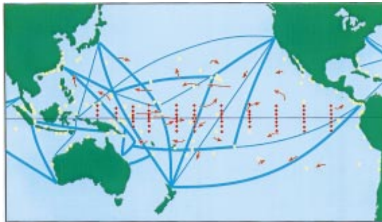
Fig. 1. The array of instruments that monitors oceanic conditions. All these measurements are relayed to stations on land, in “real time”. The blue lines are the tracks of commercial ships that deploy instruments that measure temperature to a depth of a few hundred meters. The arrows are drifting buoys that measure temperature and the winds, and whose movements yield information about surface currents. The yellow dots are tide gauges that measure sea level which depends on the average temperature of a water column. The red diamonds, buoys moored to the ocean floor, are locations where temperature is measured over the upper few hundred meters of the ocean. The red squares indicate where oceanic currents are measured.
