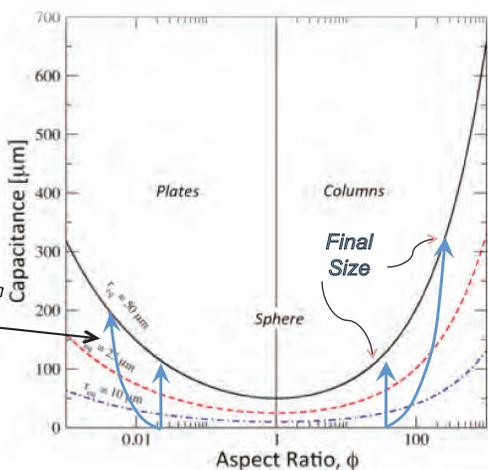
To accurately model crystal growth, must provide the link between growth and aspect ratio evolution. (Following Chen and Lamb, 1994)
