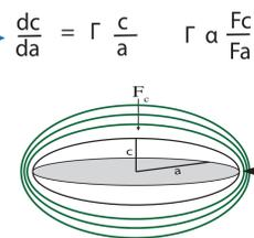
$$\frac{dc}{da} = \frac{\Gamma_c}{\Gamma_a} \frac{c}{a} \quad \Gamma_c \propto \frac{F_c}{F_a}$$
