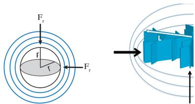
Using spheres underestimates vapor diffusion and liquid depletion
