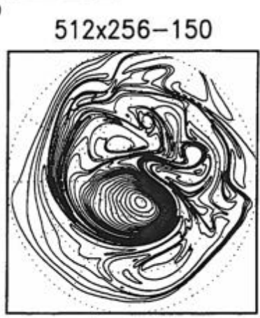
Figure 10. Polar stereographic projection (from the equator to the north pole) of the potential vorticity contours at DAY-24 in the 'stratospheric vortex erosion' test case at three different resolutions.
