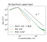
b) displays the kinetic energy (KE) spectra for upper layer flow among different models, including the fine resolution model R32 (green line), the coarse resolution model R4 (orange line), and the coarse resolution model with optimized scaling of momentum forcing R4-P (blue line).
