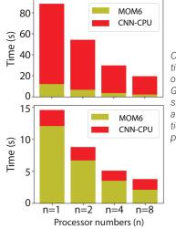
Cumulative processing time of the CNN inference on CPU (upper panel) and GPU (lower panel) alongside MOM6 simulations at the coarse grid resolution and various parallel processor counts.
