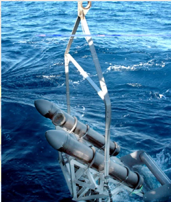
In Situ Ichthyoplankton Imaging System (70L s -1 )
