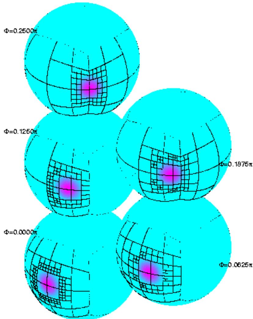
Figure 15: A cubed-sphere with embedded nests.
